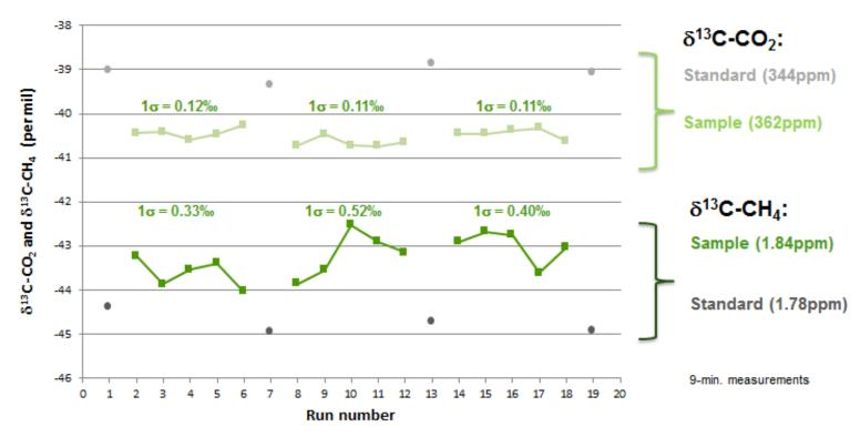
How does the SSIM2 work? When the measurement sequence begins, a 20ml sample chamber within the SSIM2 is purged and evacuated. The user then introduces 20ml of gas to the sample chamber from a bag, syringe, or other container. If less than 20ml is used, the SSIM2 can be set to dilute the sample to 20ml automatically. Note that the final concentration must be within the analyzer's dynamic range. The sample gas is then slowly injected into the analyzer cavity for an extended, stable measurement.
